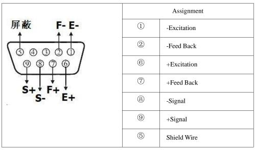
Short connect PIN 1 and 2, PIN 6 and 7 when connected a load cell with 4 wire cable;
